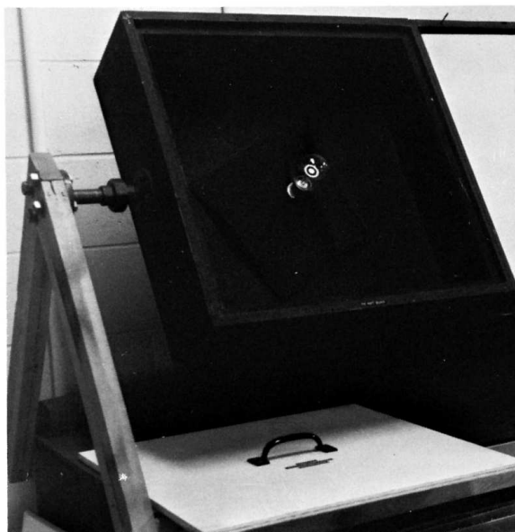
FIG. 1 Typical Unit with Pyranometer Mounted in Black Box
