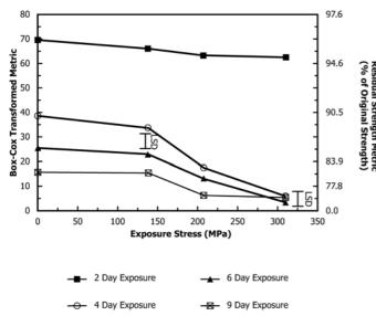
Note 1—In this case random values have been imputed for the failed specimens. Note the non-linear nature of the Box-Cox Metric (left Y-axis) as compared to the original metric (right Y-axis).
