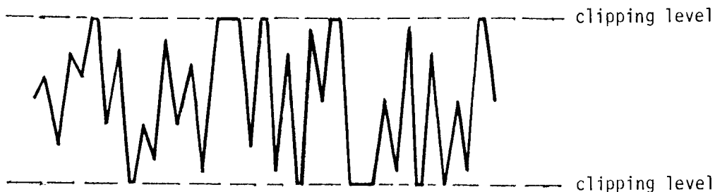
FIG. 2 Clipping of Fatigue Spectrum Loading
