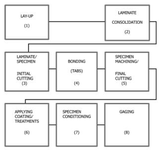
Note 1—Material identification is mandatory. Continuous traceability of specimens is required throughout the process.
