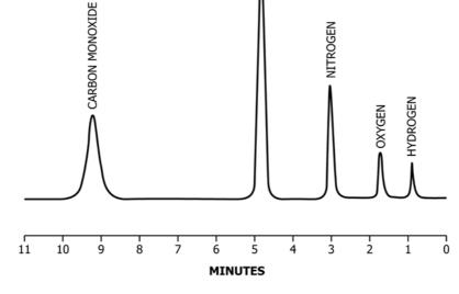
Column: 2-m by 6-mm inside diameter Type 13x molecular sieves, 14 to 30 mesh Temperature: 35°C Flow rate: 60-mL helium/min Sample size: 0.5 mL
