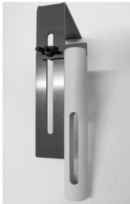
FIG. 3 In-site 1 Plating Device
