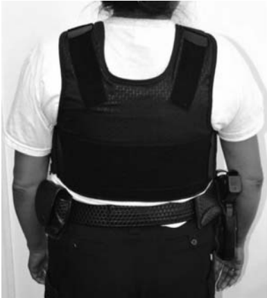
NOTE 1—The unprotected area above the top edge of vest is of concern. FIG. 11 Example Armor Showing Lack of Vertical Coverage on the Torso Back
