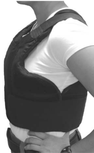
FIG. 12 Example Armor Showing Lack of Overlap on the Side and Discontinuity at Upper Side Edge of Vest
