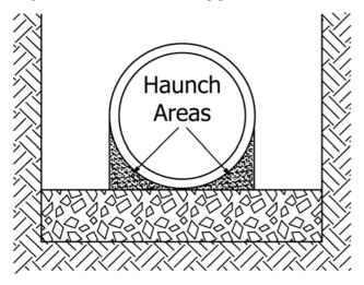
**haunching**—utilizing a shovel, spade, or other suitable tool to place and consolidate the bedding material in the haunch to (1) ensure the pipe will remain true to line and grade and (2) provide uniform circumferential support to the pipe, which is essential for the total load factor to be realized.
