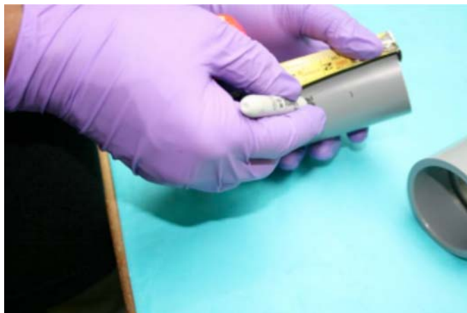
FIG. 10 Mark the socket depth on the pipe end and place a second mark 2 inches (50.8 mm) from the first mark
