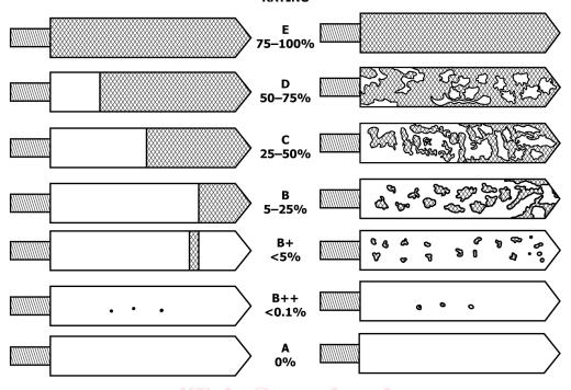
Rating shall be based exclusively on the portion of the test specimen exposed within the test fluid. Rust formed during the test has had limited opportunity to darken, and all etching or deposition of solids not removed by washing with naptha or isoctane shall be considered rust.
