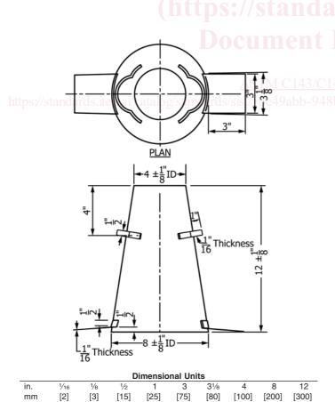
FIG. 1 Mold for Slump Test
