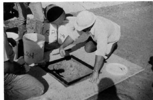
FIG. 5 Excavation of the Test Pit
