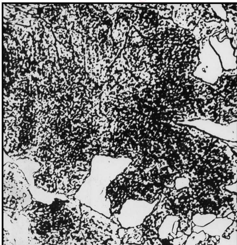
FIG. 1 Plate 1—IFI Spheroidization Rating (continued)
