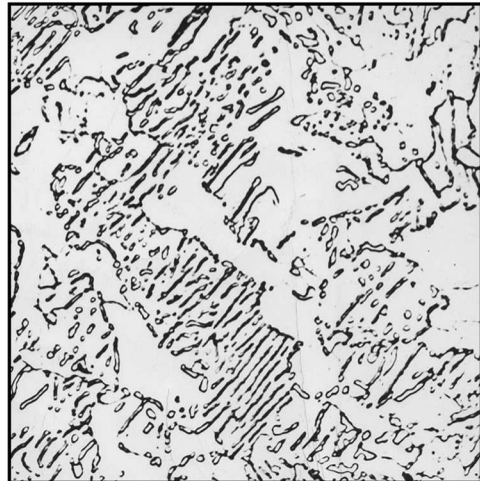
FIG. 1 Plate 1—IFI Spheroidization Rating
