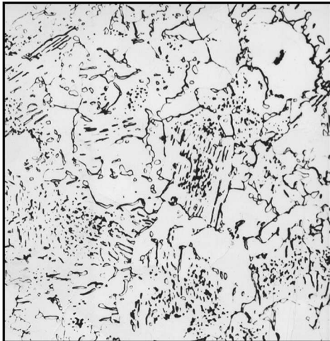
FIG. 1 Plate 1—IFI Spheroidization Rating
