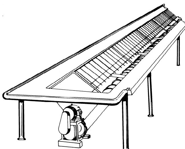
**4 conveyor, belt type** : Apparatus consisting of a conveyor belt which conveys from one point to another either grapes, or the stalks or the pressings (or marc).
