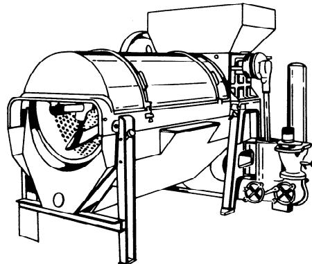
**17 juice separator** : A static or dynamic device intended to separate the juice from the grapes, which have generally been crushed, or the juice from the fermented pomace, with or without pressure.
