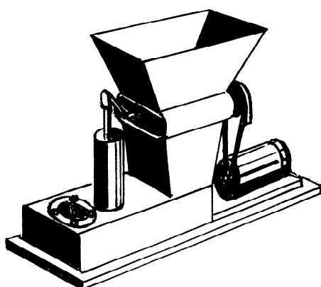
**16 crusher — stalk separator — pump unit** : A machine consisting of a stalk separator (or a crusher and stalk separator) and a grape pump.
