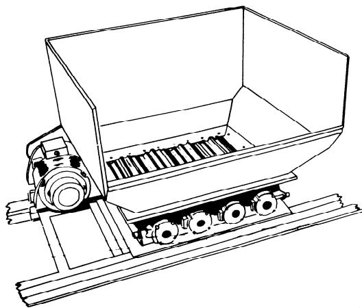
**8 crusher, cylinder type** : A crusher consisting of a set of two cylinders having a keyed or sprocketed section, revolving in opposite directions without touching, so that the grapes pass between them and burst, releasing their juice.
