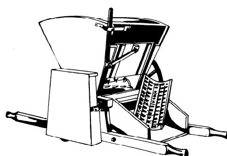
**14 grape pump** : A machine which receives the grapes and forces them into the installation through a pipe system.
