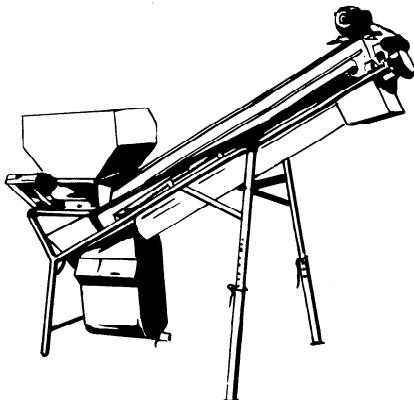
**22 juice separator, compression type** : An elevator-type juice separator, in which the screw extends beyond the outlet into a perforated drainage tube, and which may have at one end a device which exerts slight pressure on the grapes, thus increasing the degree of juice separation.
