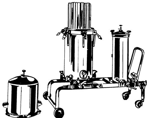
**51 filteraid filter** : Apparatus in which the filter element is composed of finely divided inert particles (Kieselguhr) held on supports.
