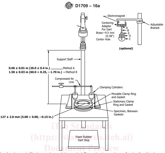
Note 1—Values for tolerances in SI units are to be regarded as standard. The numbers in parentheses reflect the allowable tolerance range of older equipment and are only provided for information and, in many cases, do not correspond directly to the tolerances in SI units. The differences are not expected to have a significant effect on the results but the dimensions in SI units shall be used in cases of dispute.
