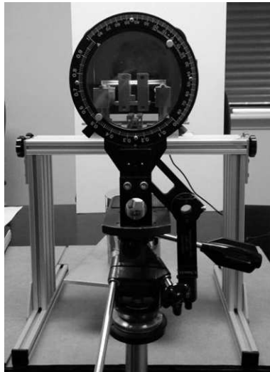
FIG. 4 Optical and Mechanical Details for Beam Method Typical Beam-Bending and Polarimeter Apparatus
