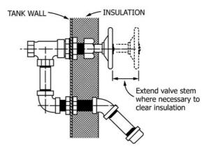
FIG. 1 Typical Submerged Sampling Device
