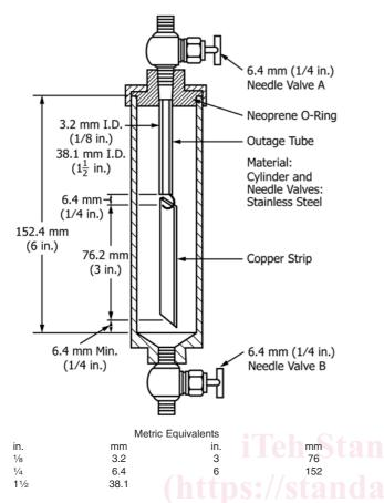
FIG. 1 Copper Strip Corrosion Test Cylinder
