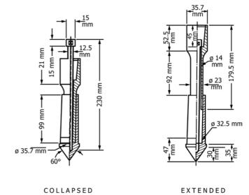
FIG. 1 Example of a Mechanical Cone Penetrometer Tip (Dutch Mantle Cone)
