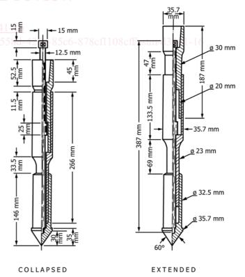
FIG. 2 Example of a Mechanical Friction-Cone Penetrometer Tip (Begemann Friction-Cone)
