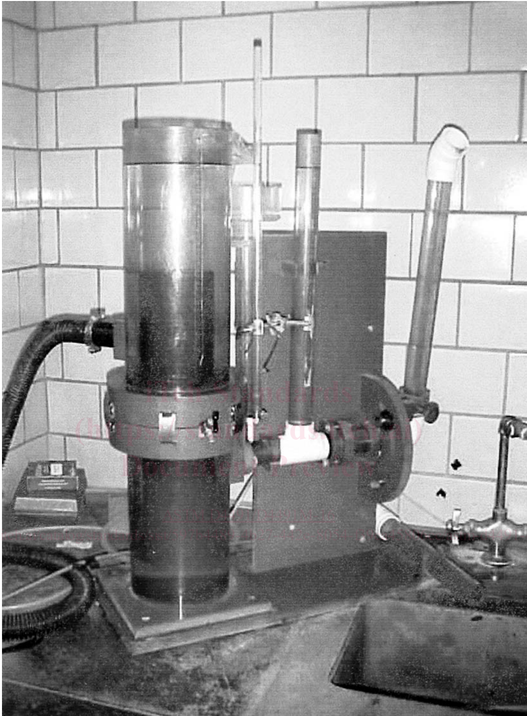
FIG. 1 Constant and Falling Head Permeability Apparatus
