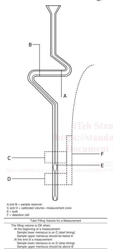
FIG. 2 Houillon Tube Schematic Diagram
