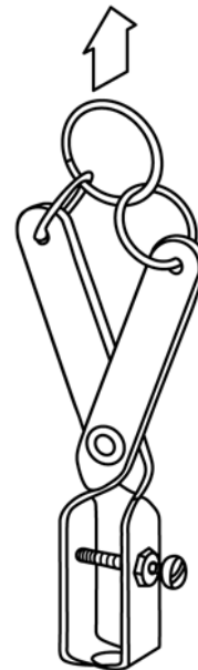
FIG. 8 Tension Test Adapter/Clamp
