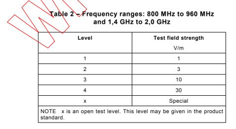
The test field strength column gives values of the unmodulated carrier signal. For testing of equipment, this carrier signal is 80 % amplitude modulated with a 1 kHz sine wave to simulate actual threats (see figure 1). Details of how the test is performed are given in clause 8.
