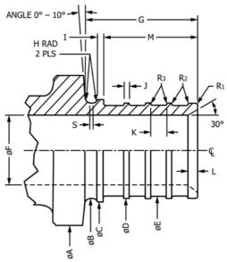
Note 1—All dimensions shall be measured with appropriate micrometers, such as pin or ball micrometers for wall thickness, and outside-diameter micrometers with flat anvils, or vernier calipers, to measure outside diameter and width of cold-expansion fittings and compression-sleeves.
