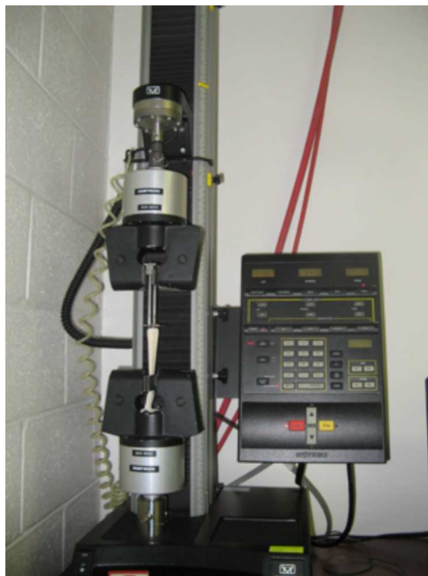
FIG. 3 Tensile Test Machine and Clamped Test Specimen
