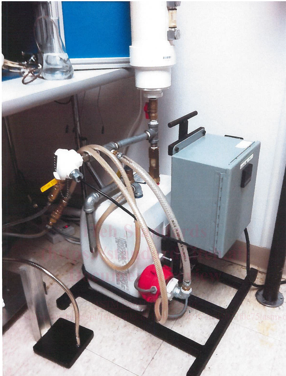
FIG. 3 Water Circulating System
