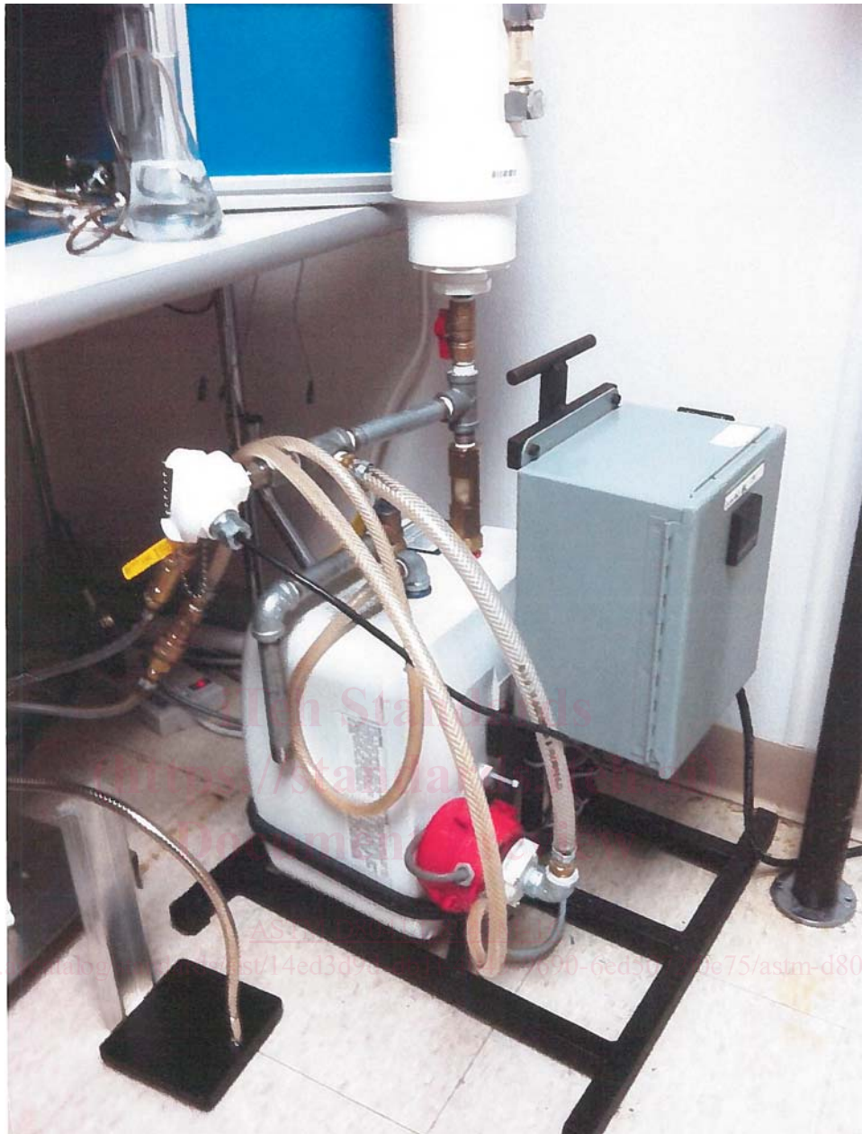
FIG. 3 Water Circulating System
