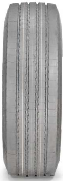
FIG. 1 Front View of the 315/70R22.5 154/150L Radial Truck Standard Reference Test Tire
