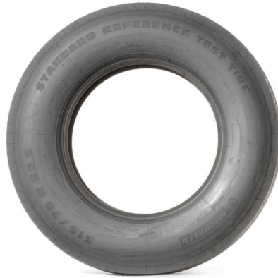
FIG. 2 Side View of the 315/70R22.5 154/150L Radial Truck Standard Reference Test Tire
