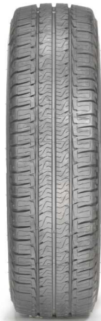
FIG. 1 Front View of the 225/75R16C 116/114S Radial Light Truck Standard Reference Test Tire
