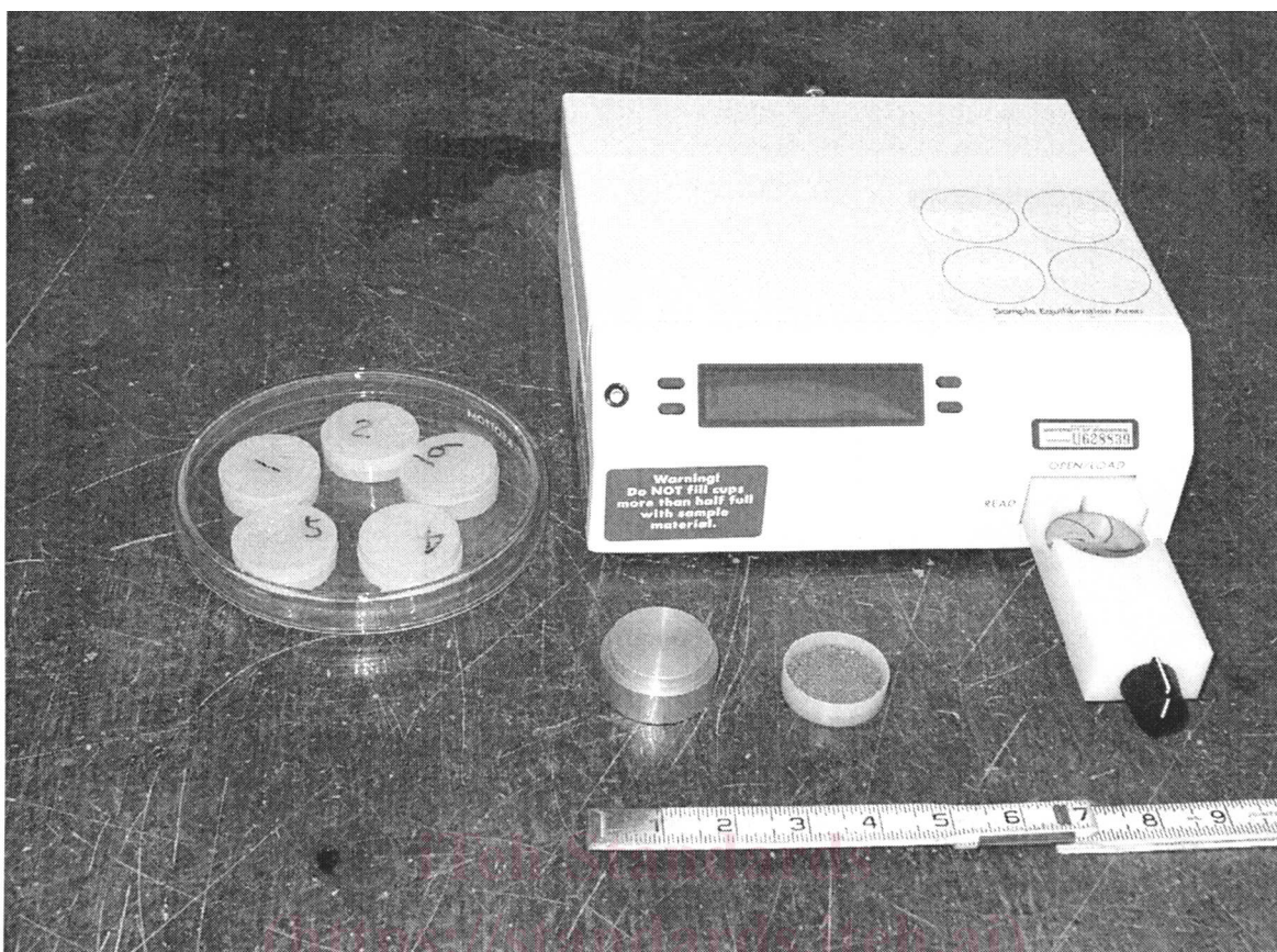
FIG. 7 Photograph of a Chilled Mirror Hygrometer With Open Sample Drawer and Specimen to be Inserted for Testing
