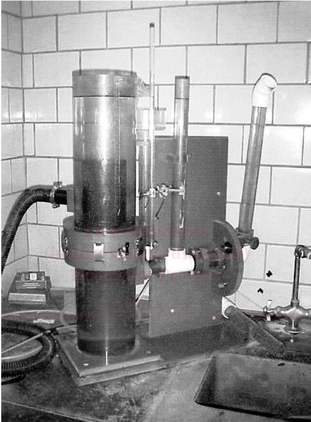
FIG. 1 Constant and Falling Head Permeability Apparatus
