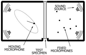
Note 1—This figure is not meant to be a design guide but is for illustrative purposes only. As an example, the room on the right has fixed microphones to measure average sound pressure level; the room on the left has a continuously moving microphone to measure average sound pressure level. Usually both rooms will have the same microphone system. The loudspeakers in the rooms generate the incident sound fields for the measurement of level differences or sound decay rates.
