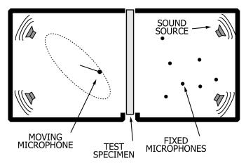
Note 1—This figure is not meant to be a design guide but is for illustrative purposes only. As an example, the room on the right has fixed microphones to measure average sound pressure level; the room on the left has a continuously moving microphone to measure average sound pressure level. Usually both rooms will have the same microphone system. The loudspeakers in the rooms generate the incident sound fields for the measurement of level differences or sound decay rates.
