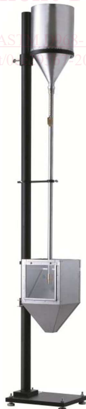
FIG. 1 Apparatus for Falling Sand Abrasion Test
