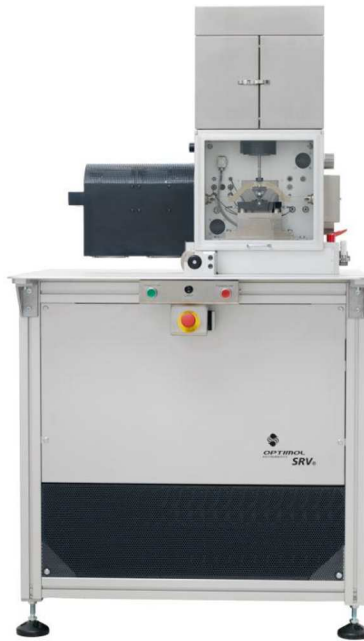
FIG. 3 SRV Test Machine (Model IV)
