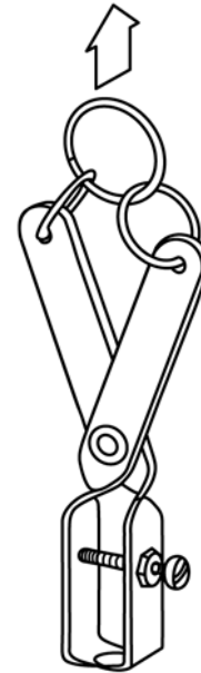
FIG. 8 Tension Test Adapter/Clamp
