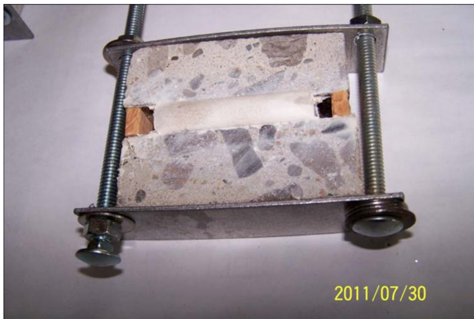
FIG. 3 Clamping Device Holding the Specimen in Compression
