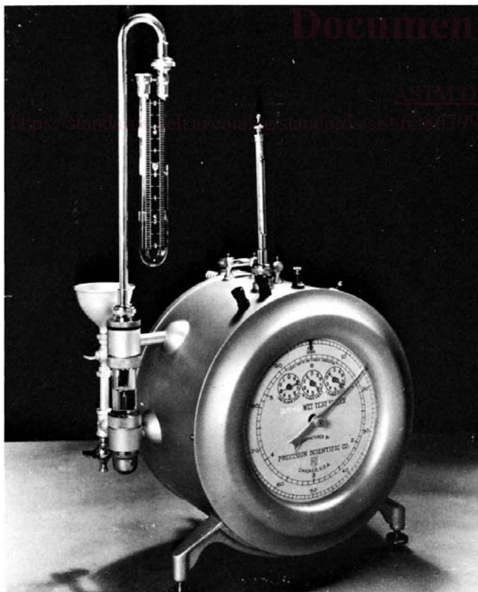
FIG. 3 Liquid-Sealed Rotating-Drum Gas Meter of 0.1 \text{ ft}^3 per Revolution Size
