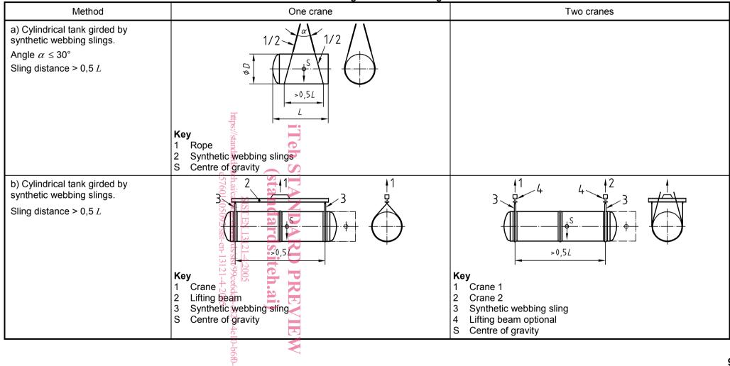
Table A.1 - Allowable lifting methods for straight vertical lift
