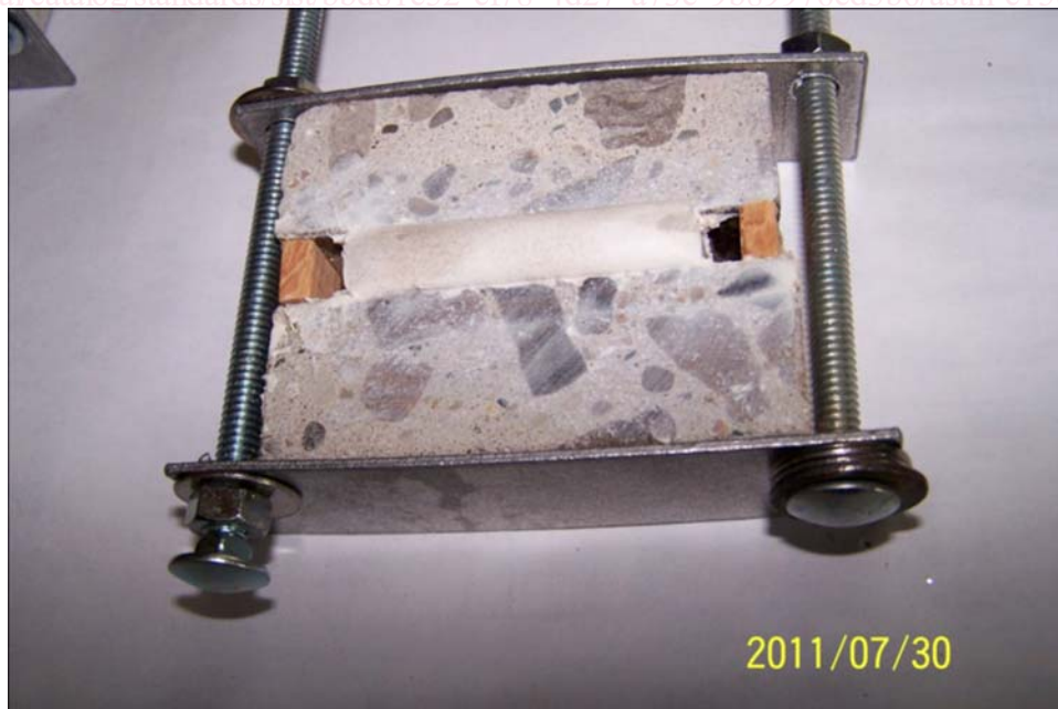
FIG. 3 Clamping Device Holding the Specimen in Compression
