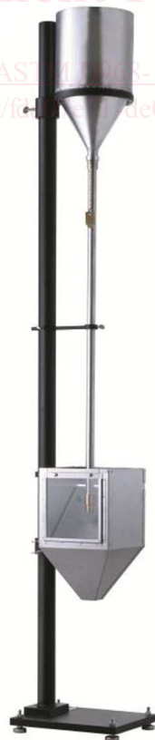
FIG. 1 Apparatus for Falling Sand Abrasion Test
