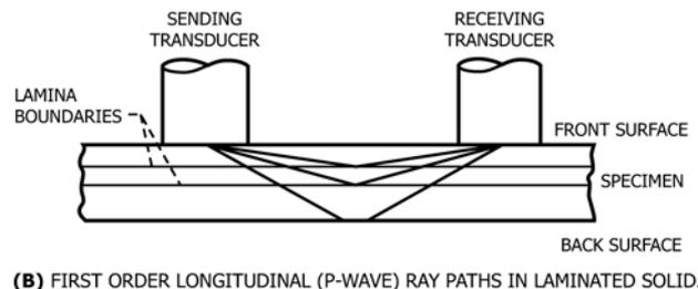
FIG. 3 Point Source-Receiver Ray Traces Illustrating the Development of AU Signals from Reflected Waves in a Monolithic and Laminated Solid
