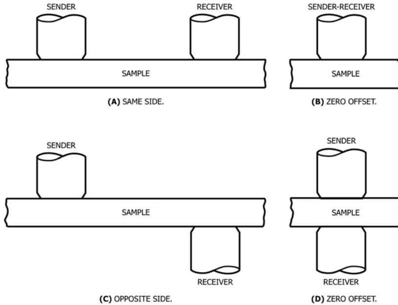
FIG. 1 Four Possible AU Probe Configurations
