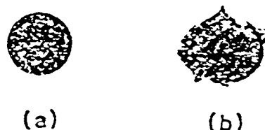
FIG. 4 Etched Areas (NaOH on Al) Showing (A) Good Gasket Fit and (B) Poor Fit Showing Undercutting of Gasket as a Result of Undertightening or Worn Gasket
