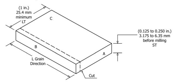
Face A is polished to .812  $\mu$ m (32  $\mu$ in.) R<sub>a</sub> or finer FIG. 1 Test Specimen
