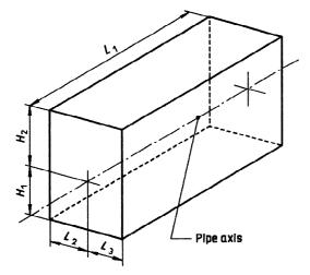
$H_1 + H_2$ ,  $L_1$ ,  $L_2 + L_3$  define the height, length and width respectively of a cuboid within which the water meter can be contained (the cover being at right angles to its closed position).
