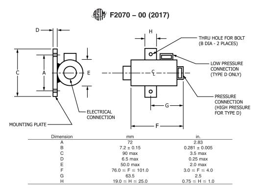
NOTE 1—Transducer housing (body) cross section is shown as circular. Any alternate cross section not exceeding 50 mm (2 in.) in width and 50 mm (2 in.) in height is acceptable.
