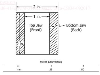
FIG. 1 Schematic Illustration of Jaw Faces for Modified Grab
