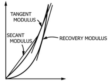
FIG. 2 Relationship Between Tangent, Secant, and Recovery Moduli for a Single Loading and Unloading Cycle
