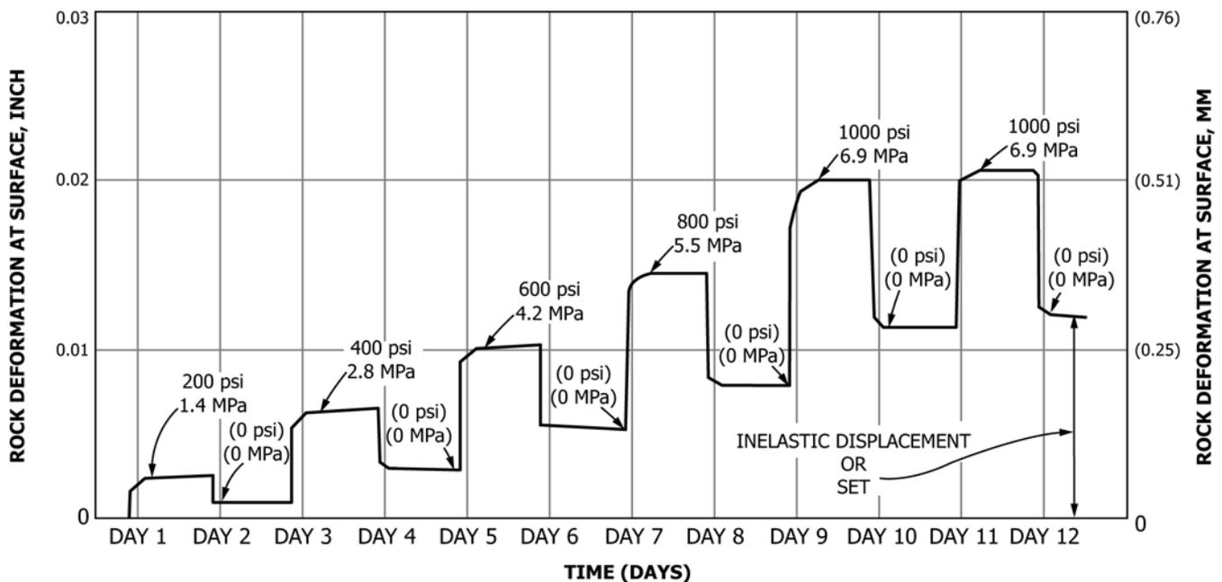
FIG. 5 Rock Deformation at Surface Versus Time Plot
